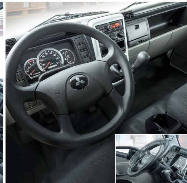
Tilt and telescopic adjusting steering wheel
